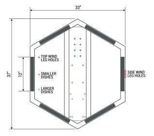
Water bins hold just under 5 gallons of water at the fill line, to equal 40 lb of water ballast. Kit weight: 30 lb
